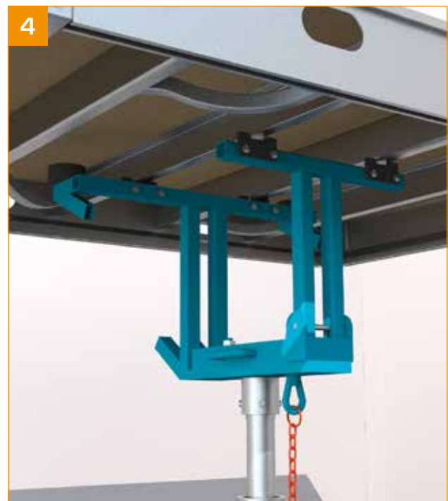
4 - The 2 central profiles of the panel support the buffers.
